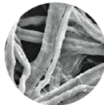
Cellulose Fiber at x500 Magnification
