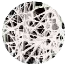
Micro-Glass Fiber at x500 Magnification
